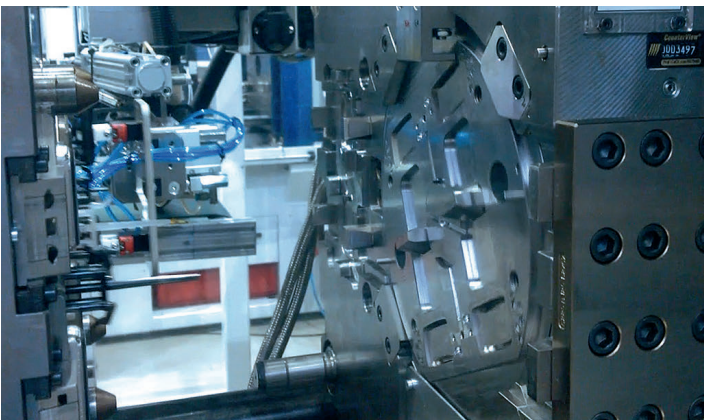
Fig. 4. The rotary plate does a 180° turn so that the freshly molded PC light guide ends up on the ejector side in station 2. There the inner contour with assembly elements is formed from black PC+ABS (© KH)
