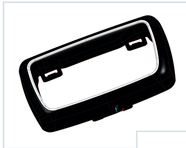
Fig. 1. The inner contour and exterior cover of the light guide (in reality both black, in the graphic green and orange for better differentiation) cannot be formed in one process (© KH)
